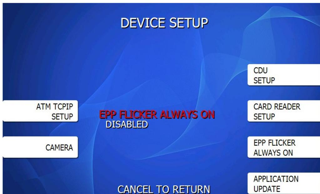
**NOTE:** If you have a Genmega G1900 model ATM, there will be a setting on the left side of the screen above for LCD Size. The options are 7" and 8" depending on which screen shipped with your ATM. If the ATM serial number begins with the letters TYPW = 7" LCD, and TYPX = 8" LCD.
